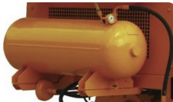
100L compressed air tank at 15 bar, that loads in 3 minutes to give a boost of pressure to the Air compressor allowing fast & effective cleaning.
