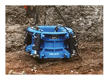
Our Quad XL cropper is designed to be used for the reduction of augured (round) piles up to 1050mm diameter. Utilising four powerful and fully synchronised rams with specially designed blades to give a superb pile cut.
