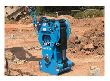
Designed to be better than the rest, and it is by some way. By utilising lighter, stronger materials we have kept the weight to 1Tonne and the dimensions small to enable easy movement around your site. Two very powerful rams ensure no pile up to 300mm will not be cut with ease by the two extremely hard wearing and fully scissoring jaws. Hydraulic control boxes ensure the two jaws operate in complete unison giving you much less trimming work at finish level.
