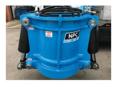
The larger Contig as with it's smaller sibling, is built with the purpose of reducing piles in a contiguous or secant wall (up to 650mm) formation where only two sides of the pile can be exposed and spaces between adjacent piles is tight.
