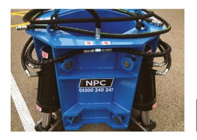
Our Quad 600 cropper is designed to be used for the reduction of augured (round) piles up to 600mm diameter. Utilising four powerful and fully synchronised rams with specially designed blades to give a superb pile cut. The cropper will also hold the cut pile section safely for removal to a designated safe area.
